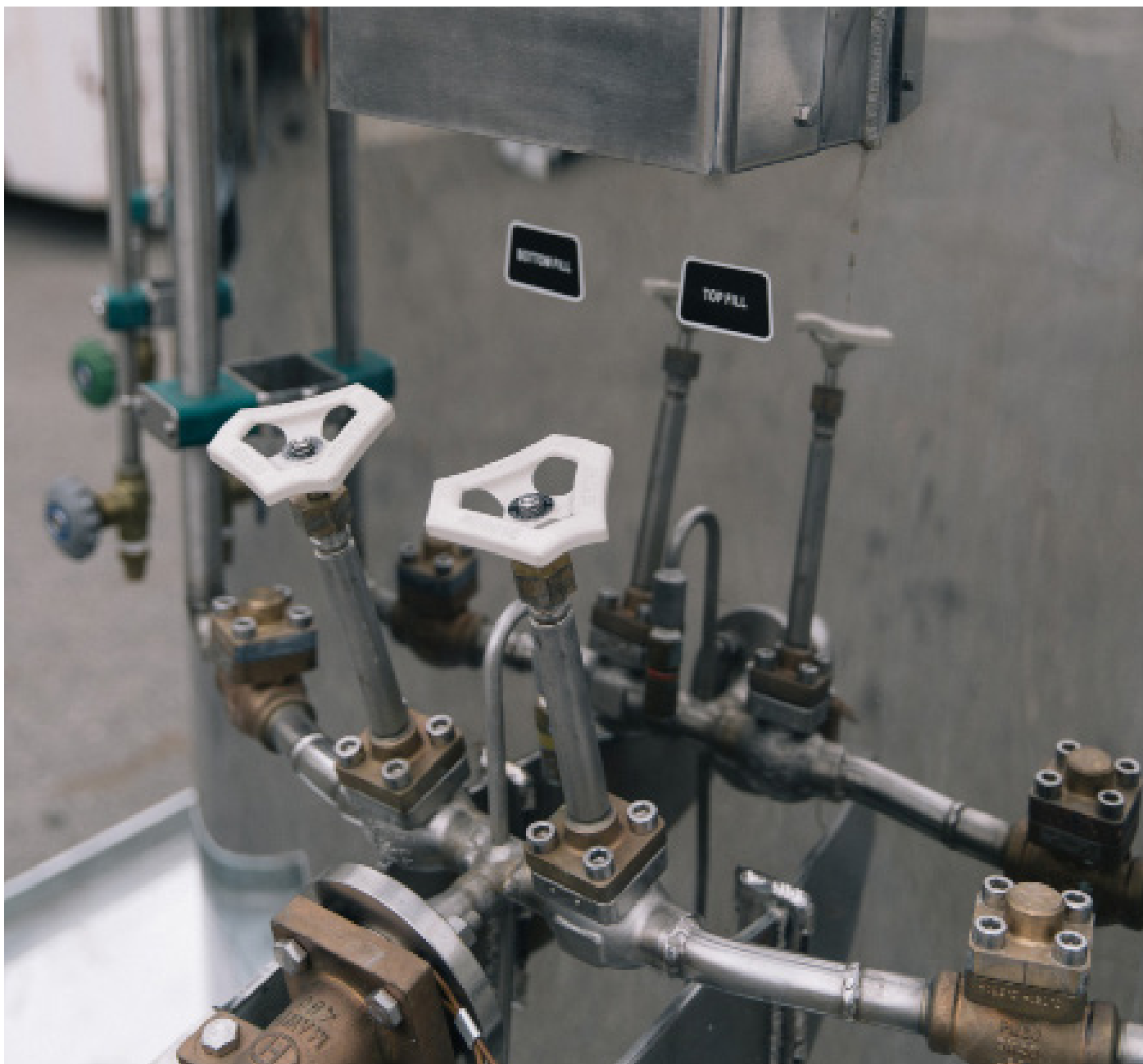
Top & bottom fill valves on the Arctic Fox 6000L tank
